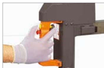
Pneumatic positioning of the mounting head
