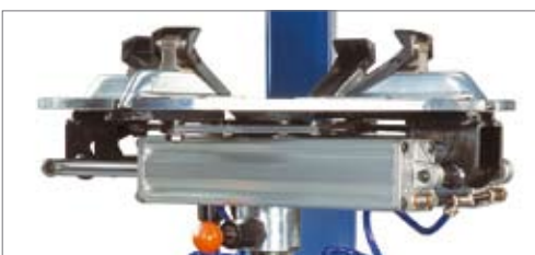
Turntable with two working heights
